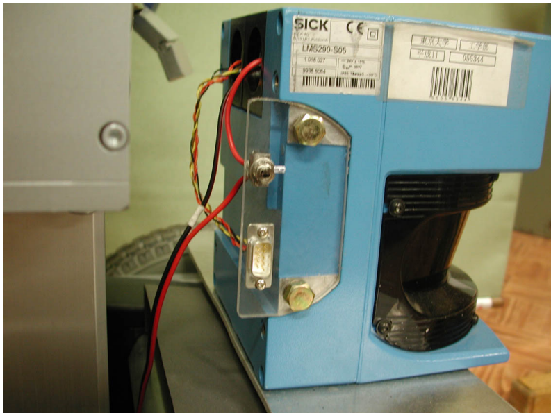
図 4.8: The switch and the connector on the acrylic board
