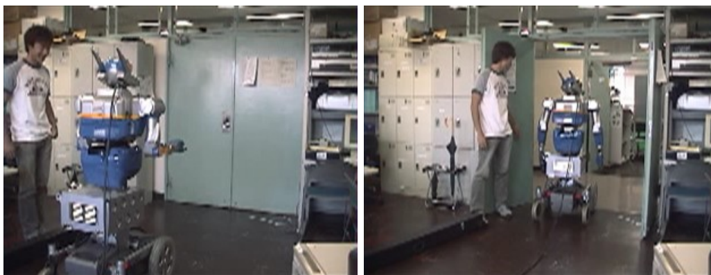
図 5.15: the experiment of waiting the door open using color recognition
