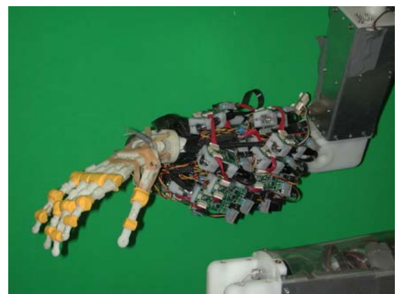
Fig. 4. A reinforceable muscle hand for Kenji
