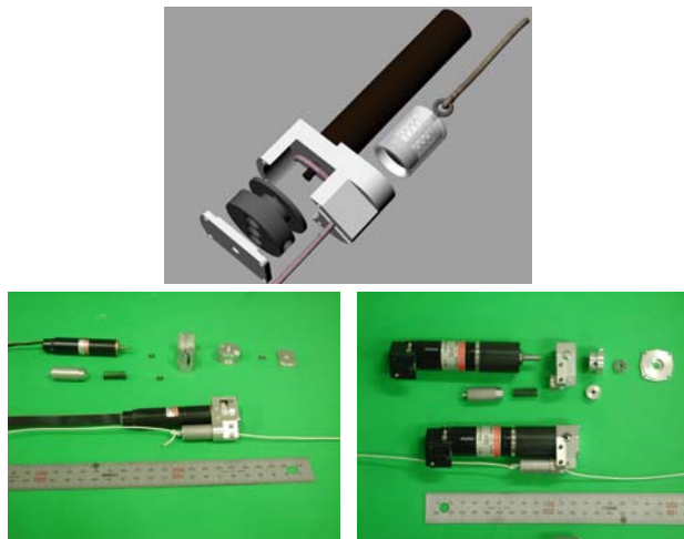
Fig. 5. Muscle units for legs. The upper figure shows the structure of a unit, the left photo shows a smaller unit using 4.5W motor, and the right photo shows a larger unit using 20W motor.
