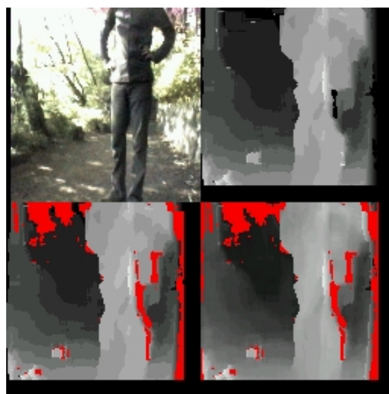
Fig. 4 Left Top: Input image, Right Top: Disparity image (brighter is closer), Left Bottom: Disparity image with consistency checking, Right Bottom: Disparity image with consistency checking and sub-pixel interpolation
