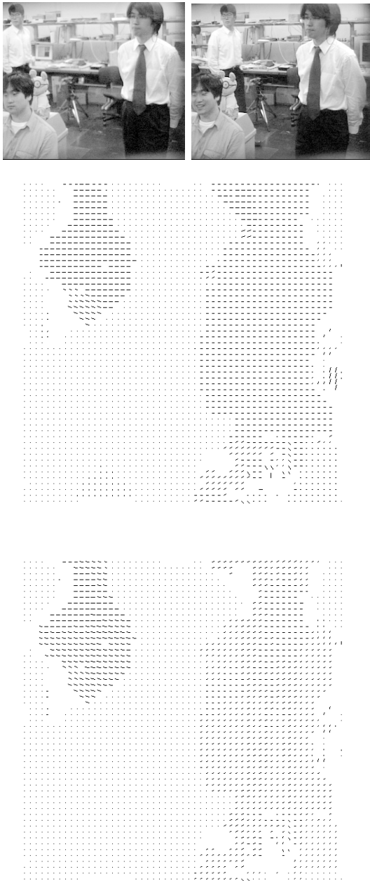
Fig. 5 Real-time optical flow generatio experimen. Top: Input image, Middle: Optical flow, Bottom: Optical flow with sub-pixel interpolation.
