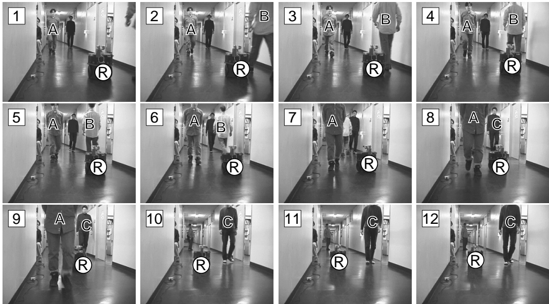
Figure 5: An experiment of moving obstacles avoidance while a robot is running.
