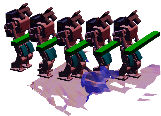
(D) Result of the path planning with an obstacle avoidance.
