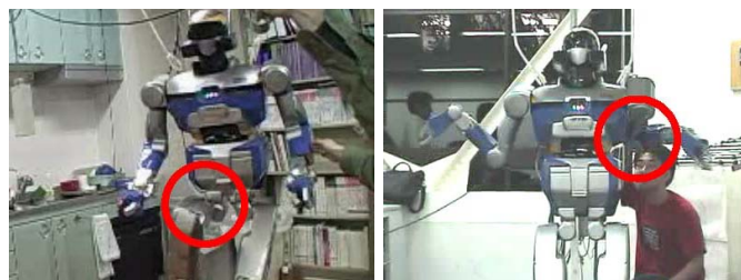
Fig. 1. Self collisions in a humanoid robot
