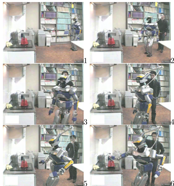
Fig.7 Play back phase: the robot uses planner for replay the taught motions
