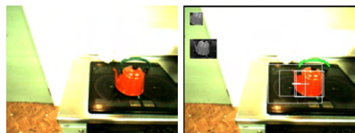
Fig.4 Image Processing for manipulation. The stereo vision calculates the position of target object.
