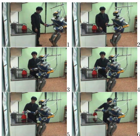
Fig.6 Teaching phase: the operator leads the robot's hand for navigating walking and manipulation.
