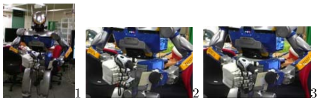
Fig.9 Use hand drill to make a hole
