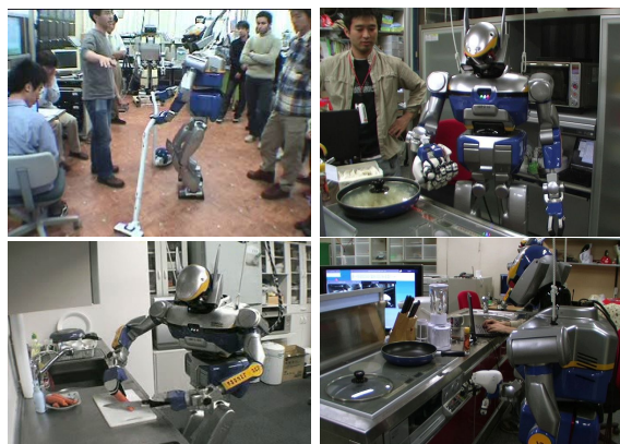
Fig.1 Some tasks by humanoid robot: Cleaning by a vacuum, cutting by a knife, pushing switches, shaking a frypan.
